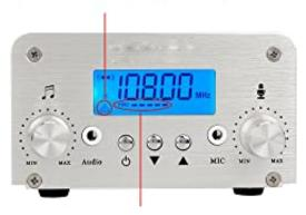
After the FWD words, there are 8-level RF power, The waitings frequency is separated by 1.9W, The Power waitings orders in 1.9W, 3.8W, 5.7W, 7.6W, 9.5W, 11.4W, 13.3W, 15W
